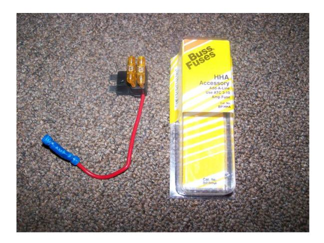
Isn't that clever? You just remove the fuse in your car's fuse box, insert this adapter and you now have to separate circuits protected by two separate fuses. The red lead would attach to the red lead of the generator. Make sure you use a fuse that is only energized when the engine is running, fuse usually marked with ign. Lettering.
