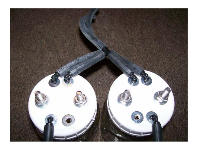
Now we want to build the exhaust system where the hydrogen gas leave the bottle and is directed to the engine.
