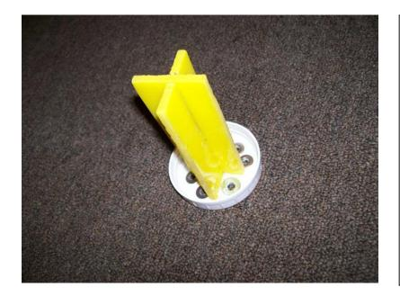
Allow the washers to dry for about twenty minutes before gluing the tower to the inside of the lid. Carefully center the tower on the lid and glue with super glue. Run plumbers goop around the edges of the tower where it meets the lid. Let dry for twenty minutes while you prepare the electrodes.
