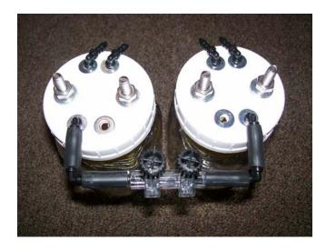
Set the two bottles with a half inch clearance between them. You are now going to build the air intake manifold.
