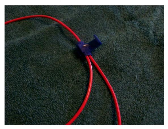
This "tap splice" allows you to splice the generator wiring into existing wiring of your vehicle. You should use this splice instead of wire-nuts. Make sure it fits 14 Gauge wiring. You insert the main power wire in one end and the original component and the generator leads in the other end. You fold the lid over and crimp with a pair of pliers. Make sure you squeeze really tight to make a good connection. I got this part at Auto Zone (part number 70026).
