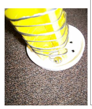
Now run the bolt up through the bottom side of the lid and thread the wire through one of the holes you drilled in the tower.
