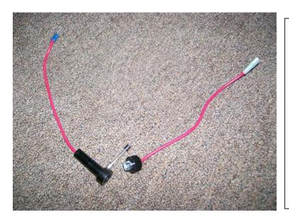
I chose to install an inline fuse right off the positive terminal at the generator even though I got my power out of the vehicles fuse box.
